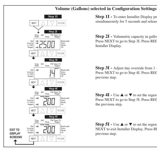
**Step 1I** - To enter Installer Display press NEXT and  $\blacktriangle$ simultaneously for 5 seconds and release.
