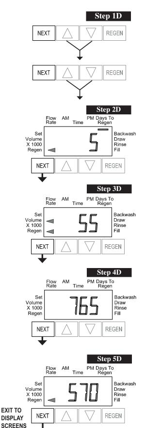
Step 1D - Press ▲ and ▼ simultaneously for 5 seconds and release. Then press ▲ and ▼ simultaneously for 3 seconds and release. If screen in Step 2D does not appear the lock on the valve is activated. To unlock press ▼, NEXT, REGEN, ▲ in sequence, then press ▲ and ▼ simultaneously for 5 seconds and release. Then press ▲ and ▼ simultaneously for 3 seconds and release.
